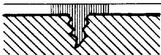
Fig. 3. Application of developer. Developer "blots" the penetrant to the surface. The defect shows up in bright red.
